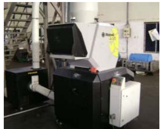
Rapid series open hearted granulator for 200 ltrs blow moulded container
