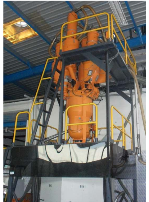
OCTOPUS: Eight components gravimetric dosing mixing system for six recipes installed with 3 nos. Multi layer film plants
