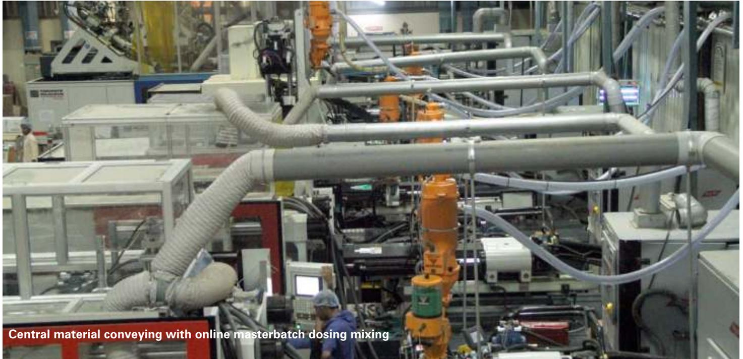
Central material conveying with online masterbatch dosing mixing
