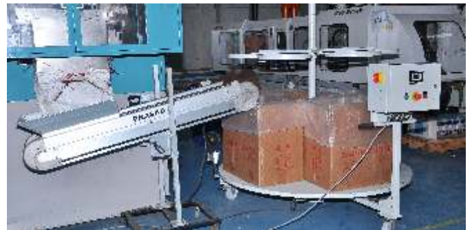
PET preform conveying and counting on high output machine
